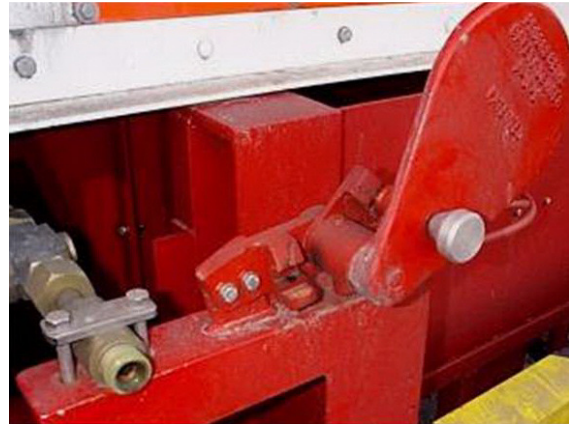
Figure B-1: Tow-away incident prevention device blocking the coupling when activated
