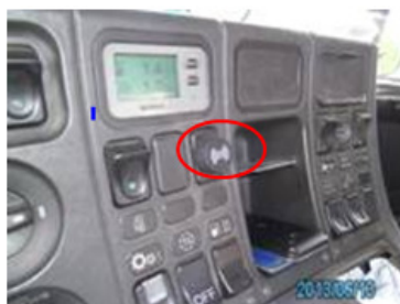
Figures B-6: In-Cab Visual and acoustic warning signs (left – visual; middle – acoustic)
